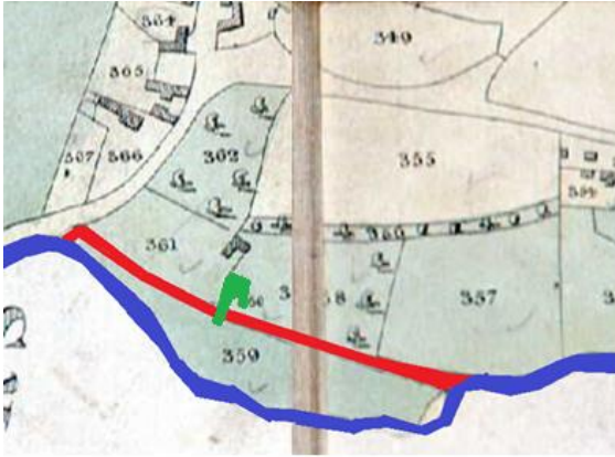
Figure 7. Field 359 identified as Water Mead (landowner John Edmonds, occupier Robert Norman) on the Netherbury tithe map. 20 On the apportionment its use is shown as meadow (2 acres, about 2 hectares). The river has been enhanced in blue, the leat in red and the mill in green. (D.H.C.)
