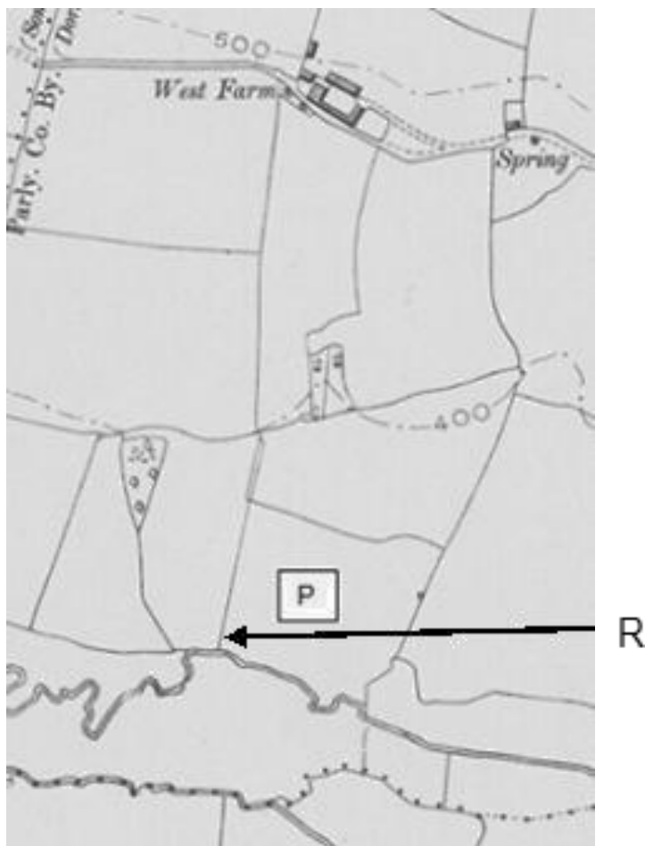
Figure 6. Enlargement from 1904 six inch OS map Dorset XX.SW. The water meadow is identified with a P. There is no evidence left on the ground to show the water meadow. From the site visit to the water meadow it is clear that it was fed from the spring. There is a ditch along the East side of the fields indicated by R. The part for the field where the water meadow was formerly has a slope to the river. The three fields on the map to the north of field P and field P have been combined into one large field in recent years. The grass was observed to be monoculture suggesting that the field has been ploughed and re-planted recently.
